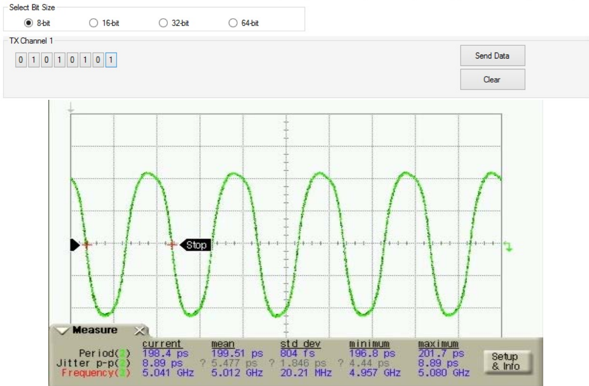
10 Gb/s Fixed TX Pattern 8-Bit 01010101 Pattern output
