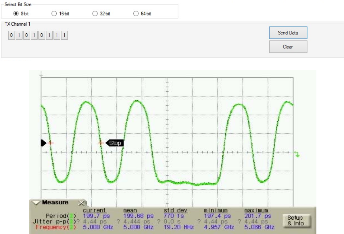
10 Gb/s Fixed TX Pattern 8-Bit 01010111 Pattern output
